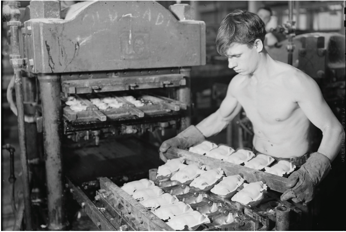
Fig. 14. Paragon Rubber molder removing dies from the press, 1930s. Photo from the National Archives and Records Administration, catalog identifier NAID 518343.
