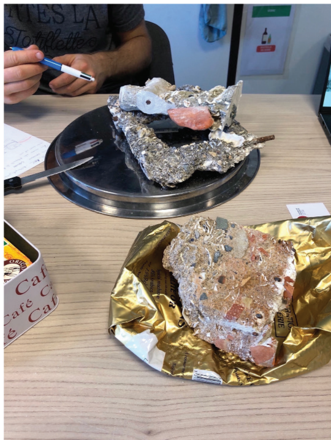
Figure 12.1. A piece of “natural concrete” produced in the harbour of Marseille. Photo by the author.
